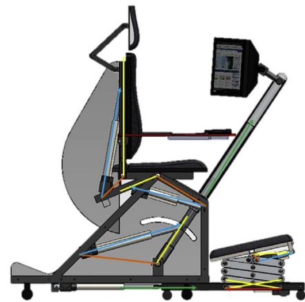
Fig. 3. Kinematic analysis of the workstation mechanisms.
