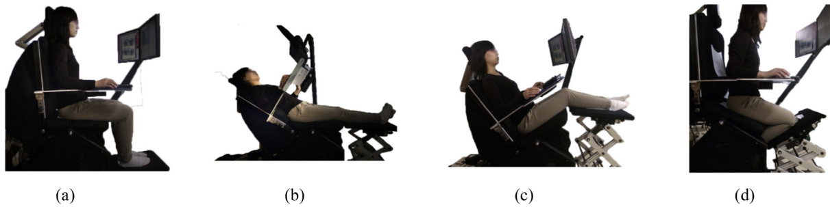
Fig. 4. Preset working positions: (a) upright, (b) lean-back, (c) zero-gravity, (d) lean-forward.
