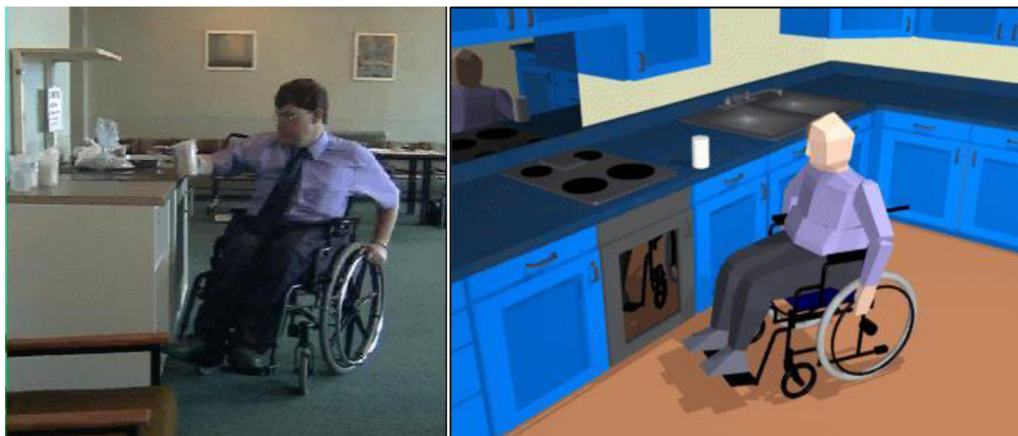
Fig. 1. Collecting task behaviour knowledge in the laboratory and simulating it in the HADRIAN digital human modelling tool. (Case et al., 2001; Porter et al., 2004).
